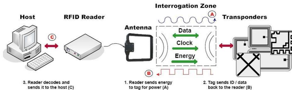
Figure 1. RFID system [11]
